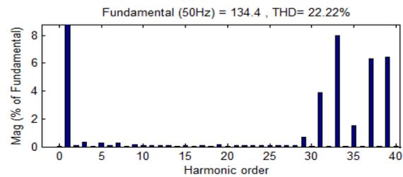
Figure 10(b). FFT plot for output voltage of UAPODPWM strategy with Sinusoidal reference
