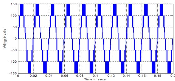
Figure 10(a). Output voltage generated by UAPODPWM strategy Sinusoidal reference
