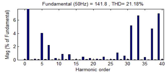
Figure 11(b). FFT plot for output voltage of UAPODPWM strategy with Trapezoidal reference
