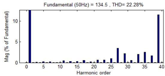
Figure 8(b). FFT plot for output voltage of UPDPWM strategy with Sinusoidal reference
