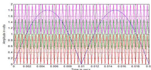
Figure 6. Carrier arrangement for UCOPWM strategy with sinusoidal reference ( $m_a=0.9$  and  $m_f=40$ )
