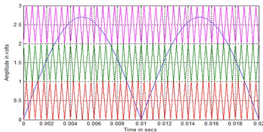
Figure 4. Carrier arrangement for UAPODPWM strategy with sinusoidal reference ( $m_a=0.9$  and  $m_f=40$ )
