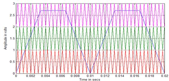
Figure 5. Carrier arrangement for UAPODPWM strategy with Trapezoidal reference ( $m_a=0.9$  and  $m_f=40$ )
