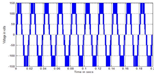
Figure 12(a). Output voltage generated by UCOPWM strategy with Sinusoidal reference
