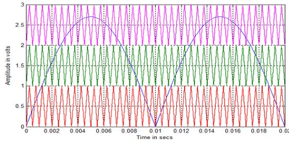
Figure 2. Carrier arrangement for UPDPWM strategy with sinusoidal reference ( $m_a=0.9$  and  $m_f=40$ )
