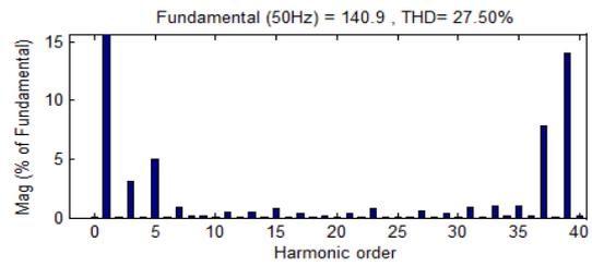
Figure 12(b). FFT plot for output voltage of UCOPWM strategy with Sinusoidal reference
