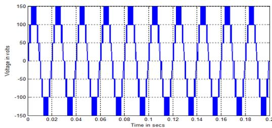
Figure 8(a). Output voltage generated by UPDPWM strategy with Sinusoidal reference
